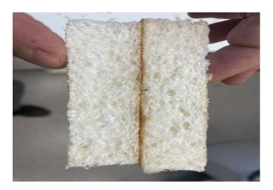
We at FOAMO developed a radical new green technology where 100% of the materials that FOAMO uses are derived from renewable natural resources. Our secret is the use of cellulose, the most abundant renewable material on earth. With it, we create a foam with a porous structure that makes it incredibly lightweight and able to absorb the impact of your foot comfortably.
